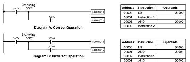
If, as shown in diagram A, the execution condition that existed at the branching point cannot be changed before returning to the branch line (instructions at the far right do not change the execution condition), then the branch line will be executed correctly and no special programming measure is required.
